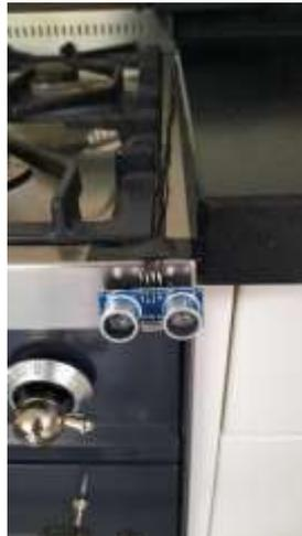
Figure 43: Ultrasonic sensor
