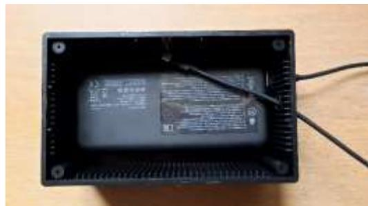
Figure 39: Inside hub with power bank
