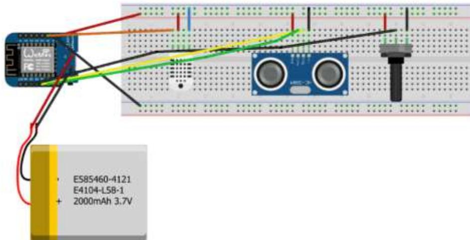
*Figure 8: Fritzing drawing hub*
