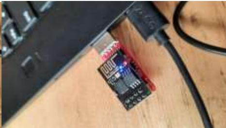
Figure 18: ESP01 Testing blinking
